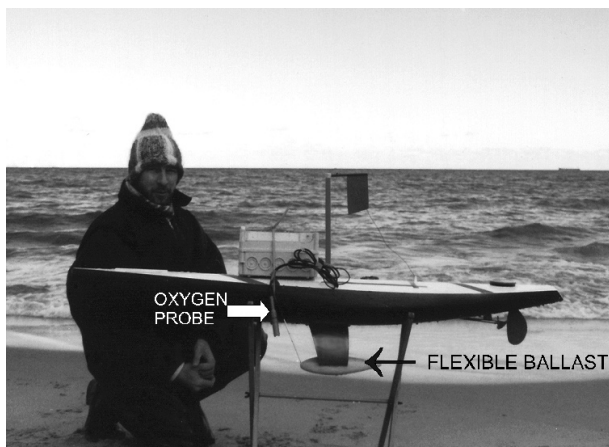
Photo 1. Radio-operated ship with deployed oxygen and water temperature probes.
